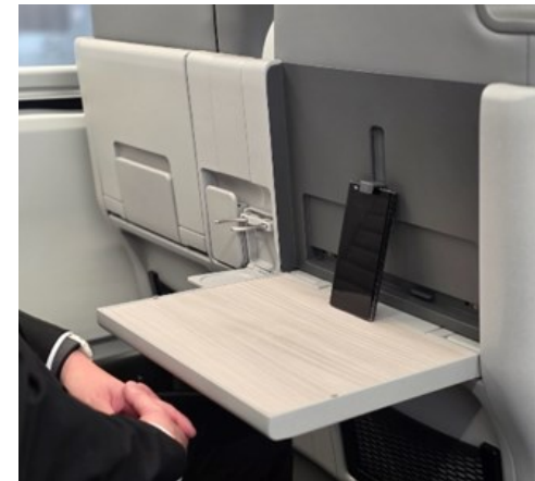
Cup holders are included on seatbacks between the normal tray tables; those tables, when folded down, reveal a cell-phone holder. Rip Watson
