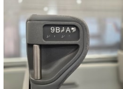
A safety feature of the Airo seats is a grab handle in each headrest along the aisles.
