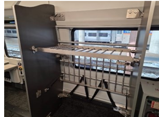
Cars include baggage racks as well as space above seating areas. Some trainsets will include compartments for checked baggage. Rip Watson
