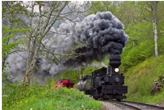
The one remaining original Cass engine, three-truck Shay No. 5, heads up a freight just below Whittaker during Railfan Weekend 2014. Built for the Greenbrier & Elk River Railroad in 1905, it is the second-oldest Shay in operation.
