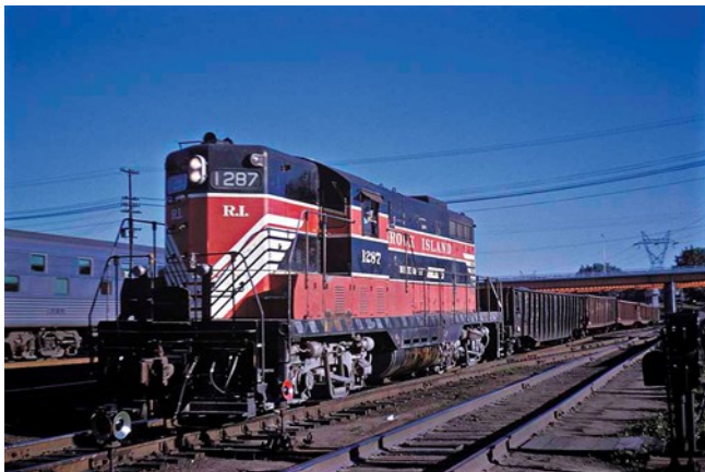
Rock Island's early EMD Geeps were delivered in an eye-catching red-and-black scheme with "Route of the Rockets" lettering on the long hood. Here GP7 No. 1287 works at St. Paul in 1961. J. David Ingles photo
