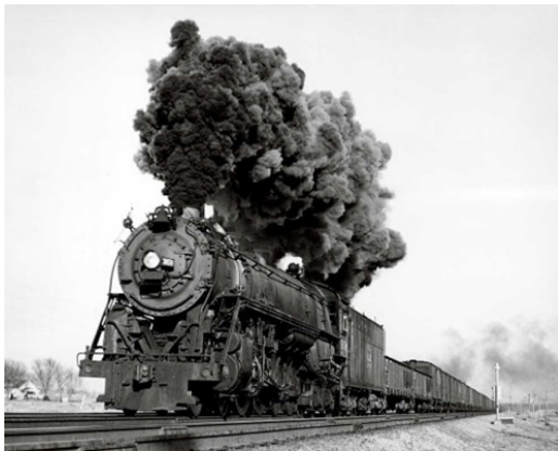
Rock Island had a fleet of 85 Northern (4-8-4s), largest in the country. Here, No. 5058 leads a west-bound freight near Lawrence, Kan., in January 1952. Robert P. Olmsted Collection, American Heritage Center, University of Wyoming
