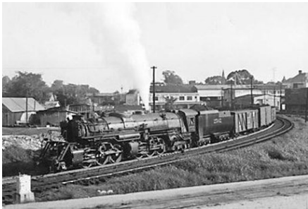
One of Seaboard Air Line's high-speed, twin smokestack 2-6-6-4s – the largest steam engines on the railroad's roster – charges out of Raleigh, N.C., with a freight in 1941. Homer R. Hill
