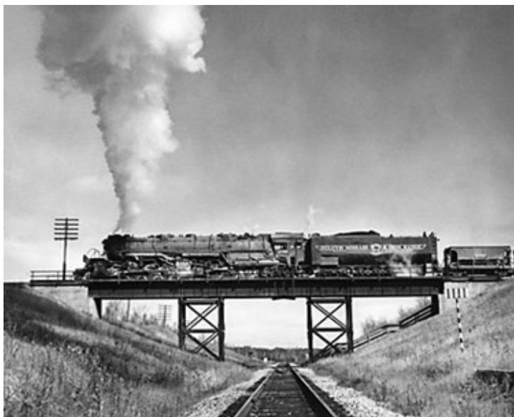
Duluth, Missabe & Iron Range 2-8-8-4 No. 236 hauls an empty ore train north out of Two Harbors, Minn. DM&IR's Yellowstone were equipped with all-weather cabs and centipede tenders. Franklin A. King
