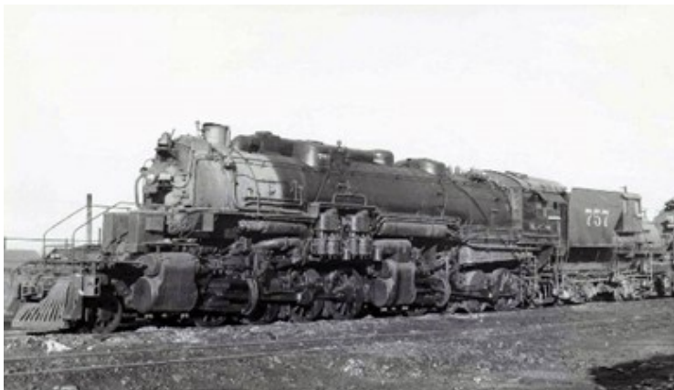
Kansas City Southern 2-8-8-0 "Big Mallie" #757 (G-2), manufactured by Alco's Brooks Works in 1924. Like most roads, the KCS found these satisfactory in drag service stating the G-2's could pull 2,700 tons "...over a ruling grade of 1.5% southbound and 1.35% northbound."
