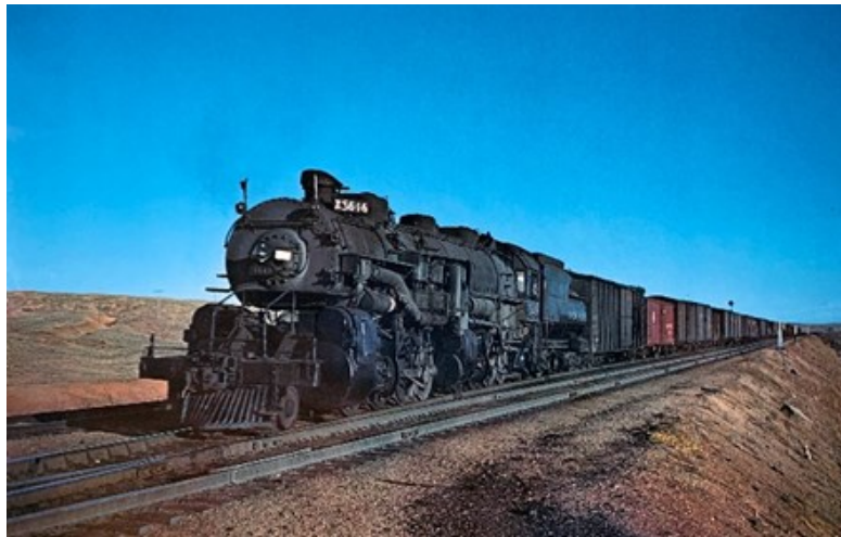
A Union Pacific publicity photo featuring 2-8-8-0 "Bull Moose" #3646 with a freight extra on Wyoming's Sherman Hill (between Cheyenne and Laramie) during the early 1940's. The 2-8-8-0's were built as Mallet's but later converted to simple expansion between 1936-1944. Author's collection.
