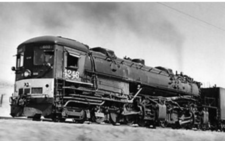
Southern Pacific cab-forward 4-8-8-2 No. 4246, a 1942 Baldwin, races through western Nevada. Robert Hale
