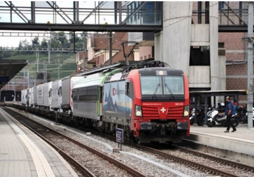
An RAlpin “Rolling Highway” train pauses in Spiez, Switzerland, for a crew change on Sept. 16, 2024. Note the sleeping car immediately behind the locomotive. AmeriStarRail is proposing similar service for trucks as part of its “Transcontinental Chief” plan. David Lassen
