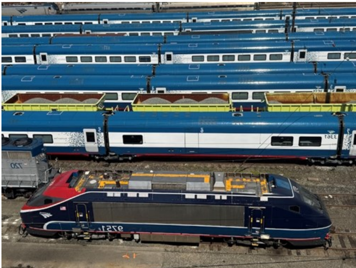
Seven Next Generation Acela trainsets and an HHP-8 locomotive converted to a cab car are spotted at Amtrak's Philadelphia coach yard on June 25, 2025. Keith Fender
