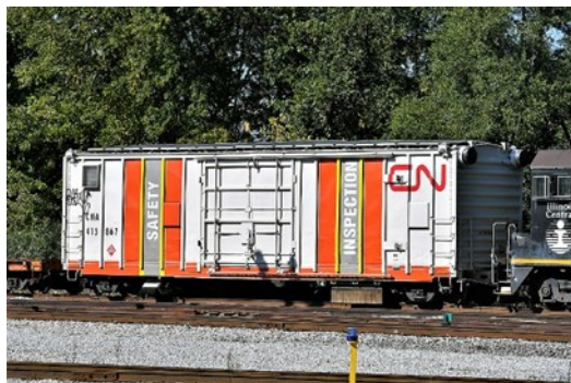
This car is part of Canadian National's Autonomous Track Inspection Program. Craig Walker
