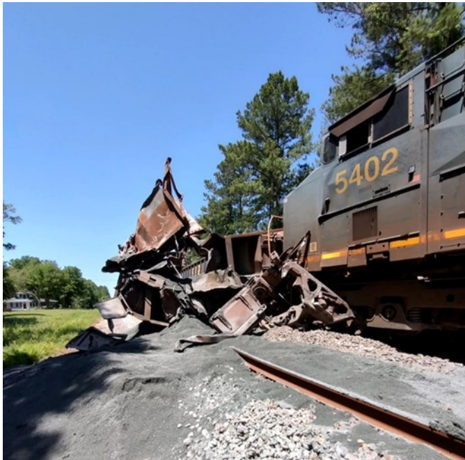
An improperly lined switch led to this 2024 collision between CSX trains in Folkston, Ga., the NTSB has determined. Charlton County Sheriff Robert Phillips
