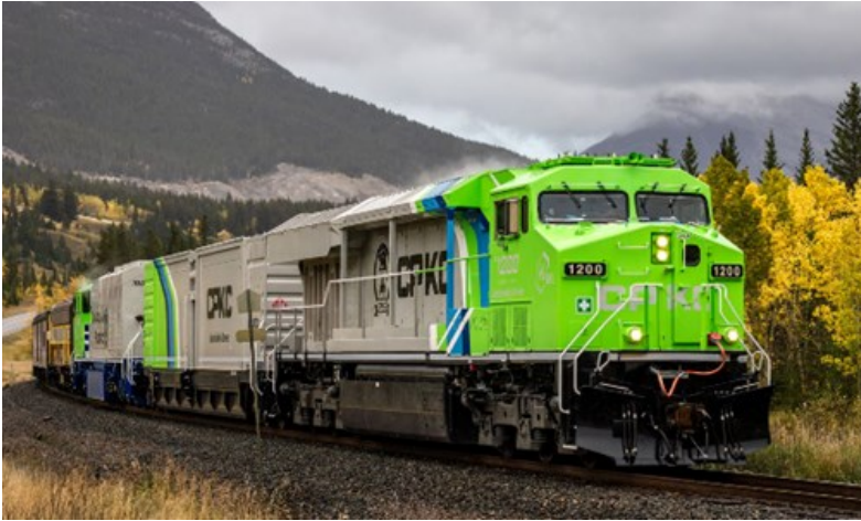
CPKC's first line-haul hydrogen locomotive, with its fuel tender, began testing in September 2024. CPKC
