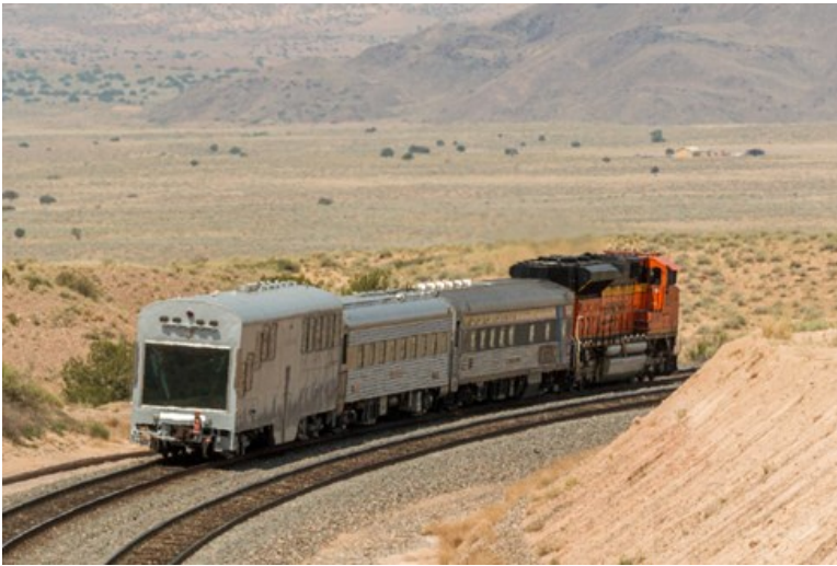
BNSF Railway uses autonomous and staffed automatic track geometry inspection cars. Here, a staffed train inspects track-age. BNSF Railway
