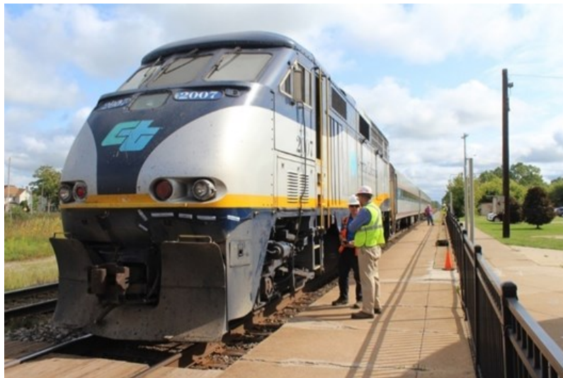
Workers examine a shunt antenna on a test train at Durand, Mich., on Sept. 13, 2023. Bob Johnston
