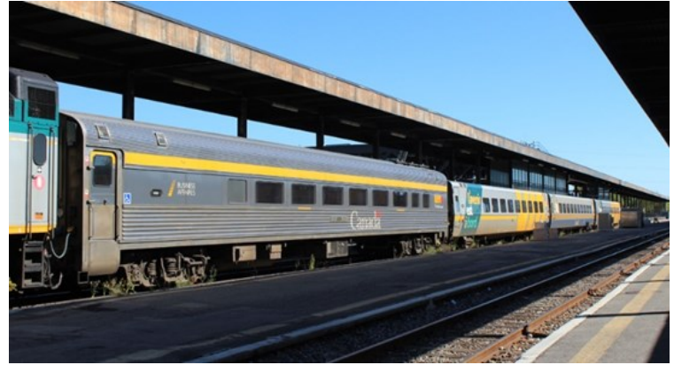
A Budd-built HEP-2 coach and three "Light Rapid Comfortable" cars await departure from Ottawa to Toronto on Sept. 30, 2024. VIA has routinely operated the LRCs in four-car sets for decades without incurring loss-of-shunt incidents. Bob Johnston
