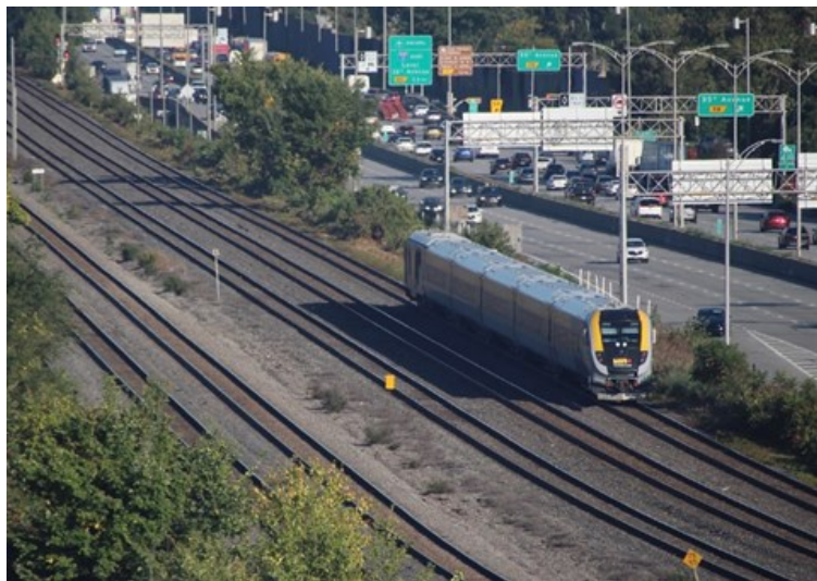
A Venture trainset handles Ottawa-bound VIA No. 37 approaching the Dorval, Quebec, station west of Montreal on Sept. 30, 2024. Canadian National has imposed axle-count restrictions on Venture equipment, reportedly because of issues with activation of grade-crossing signals. Bob Johnston
