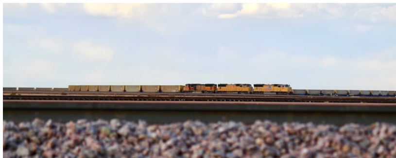
With the tail end of the 6,325-foot train still rolling around the 6-degree curve at the north end of the FAST loop, the head end of the MxV Rail test train negotiates the 6-degree reverse curve. In the foreground: The outside rail of the 5-degree curve at the loop's south end, the reverse loop track that's under construction, and the loop's access track. Bill Stephens
