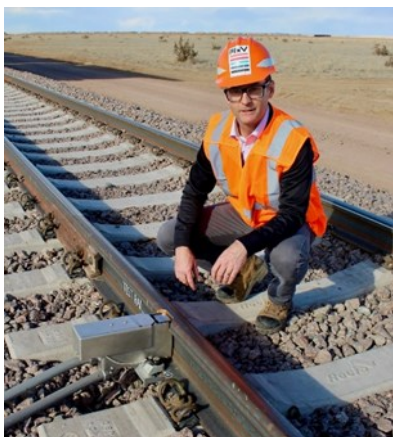
Scott Cummings, MxV Rail's assistant vice president of research and innovation, shows off an Innerspec Technologies, Inc. prototype ultrasonic cracked wheel detector at the FAST track loop in Pueblo, Colo. Bill Stephens
