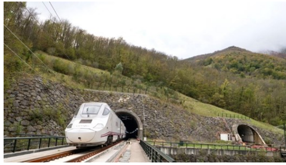
A RENFE Class 130 Alvia train exits the Pajares Base Tunnel. This type of train will be used for passenger service; it can change gauge and voltage, overcoming the new line's operating complexities. Courtesy ADIF AV
