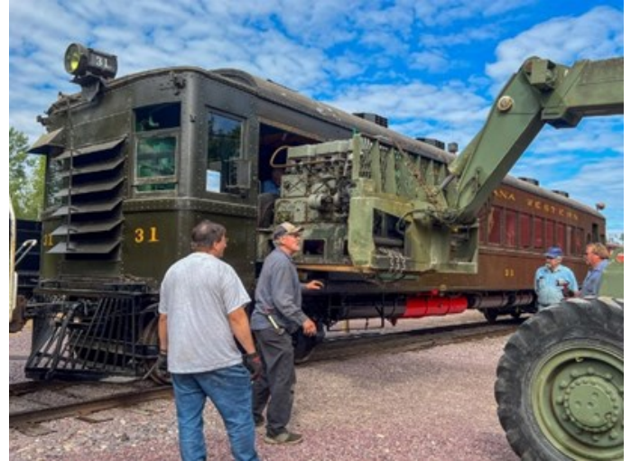
The Winton engine is removed from the railcar for shipment to FMW Solutions for disassembly and assessment. FMW Solutions
