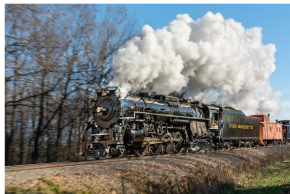
Pere Marquette No. 1225 rounds a curve near Carland, Mich., while pulling the North Pole Express excursion on Nov. 18, 2023. The Berkshire-type 2-8-4 is fresh from a wheel and running gear rebuild along with a recent repaint.
