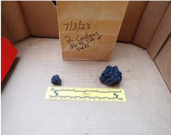
Two possible carbon particles recovered from the origin area of the Tunnel 5 Fire. Wash. DNR photo
