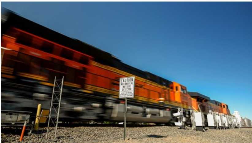
A BNSF train passes through a wayside detector array. BNSF photo
