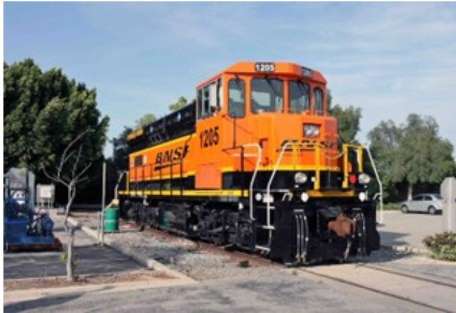
BNSF's HH20B hydrogen locomotive test unit, No. 1205, in Los Angeles in 2010. The locomotive has been donated to the Oklahoma Railway Museum. David Lustig
