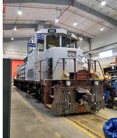
No. 1205 during its conversion to hydrogen power at BNSF's shops in Topeka, Kan., on Dec. 9, 2008. David Lustig
