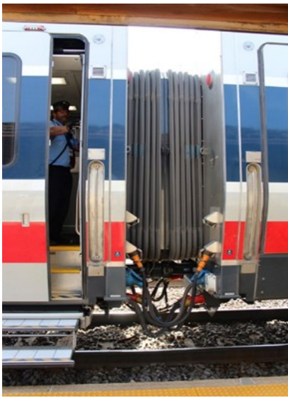
The semi-permanent coupling of the 1B coach on the left and the business class/coach on the right means they always operate in pairs. Bob Johnston
