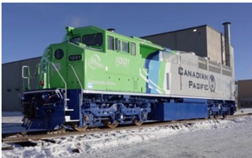
A capture from a Canadian Pacific video shows the railroad's first hydrogen fuel-cell locomotive. Its second unit, a GP38, is set to roll under its own power for the first time this month. Canadian Pacific
