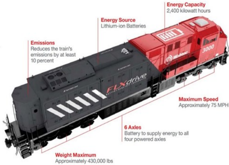
A diagram shows features of the Wabtec FLXdrive battery-electric locomotive. Wabtec
