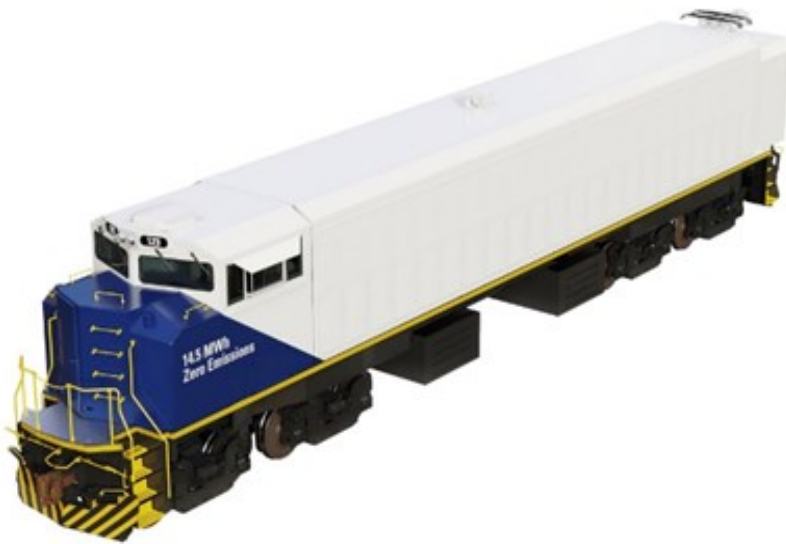
A rendering of a 14.5 megawatt-hour EMD Joule locomotive. Progress Rail
