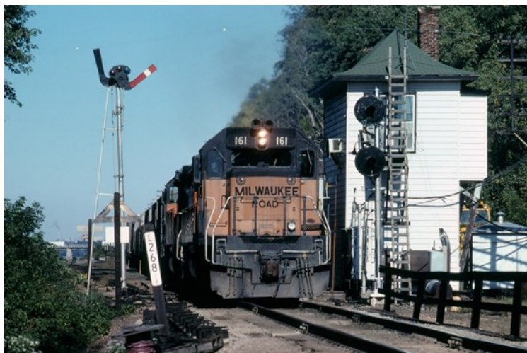
Milwaukee Road SD40-2 diesel locomotive 161 on a freight east out of St. Paul passes St. Croix Tower at Hastings, Minn., in 1984. Steve Glischinski photo
