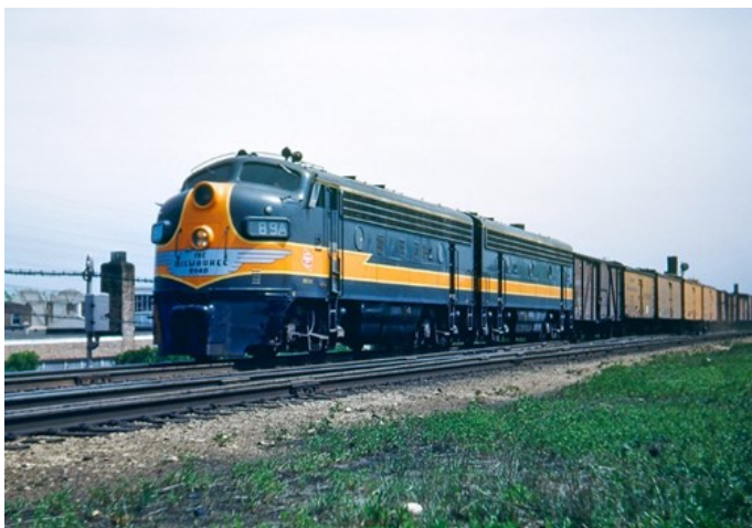
Dressed in a short-lived paint scheme for Milwaukee Road freight units, two nearly new F7 diesel locomotives lead a freight in Chicago around 1950. Robert A. Cafilisch photo
