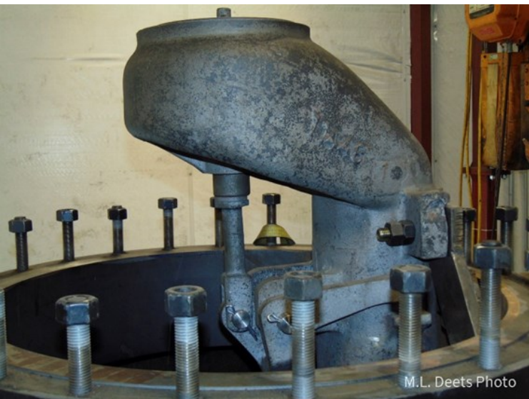
1385's throttle, located inside the steam dome.
