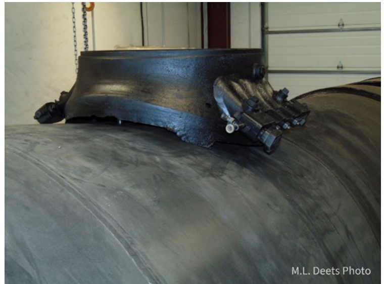
Installed sand dome. One of the new studs is visible
