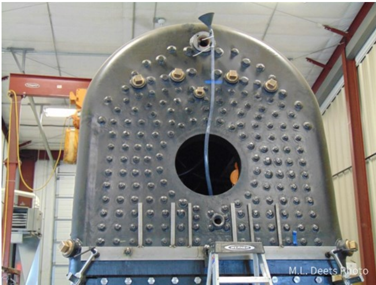
Water-filled tube coming out of firedoor and attached to backhead
