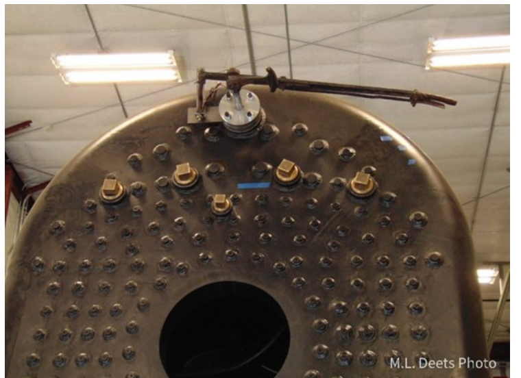
Throttle lever attached to backhead.
