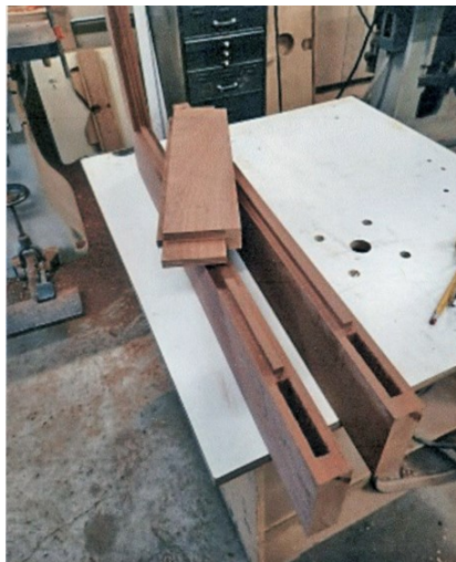
MCRM 2022 JAN 2 One of the new Soo Line #203 cupola window frames
