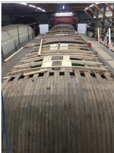
MCRM The LS&I #64 upper roof with the new carlines and blocking installed
