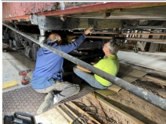
MCRM Randy and Bill working on the hand brake system under the DULUTH
