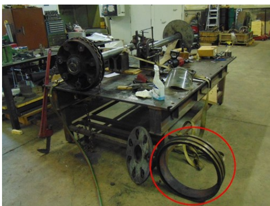
This photo from February 2017 shows 1385's disassembled piston. One of the bull rings is circled. M.L. Deets photo
