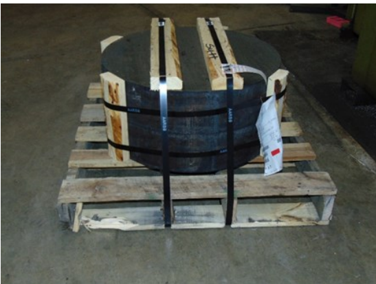
Two cast iron blanks which will become C&NW #1385's piston and valve bull rings. M.L. Deets photo
