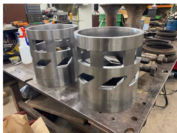
The valve cage is a hollow cylindrical wear element that is used as both a guide for the valve as well as the outer sealing surface for the valve so it can route both the live steam and exhaust steam to the proper places. The valve packing rings form the inner sealing surface and slide back-and-forth in the valve cage as the valve is moved. C&NW 1385's new valve cages stand ready to be installed into the steam chests. Steve Pahl photo.
