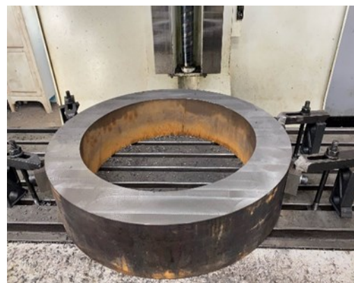
One of the cast iron "blanks" for the new piston bull rings, shown after being water jet cut to rough dimensions. Further machining is required. Steve Pahl photo.
