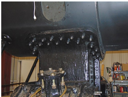
Outside view of bolts securing the smoke box to the cylinder saddle. M.L. Deets photo.
