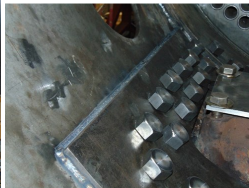
Detail view of the seal weld and bolts along the bottom of C&NW 1385's smoke box. M.L. Deets photo.
