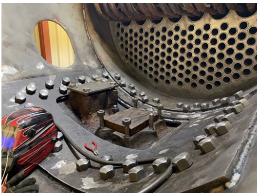
50 custom-made tapered bolts now help secure the smoke box to the cylinder saddle. Steve Pahl photo.
