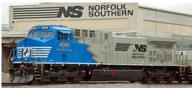
Norfolk Southern GE (now Wabtec) Dash-9 conversion to an AC44C6M type from DC to AC in 2015. Photo: Mike Ray
