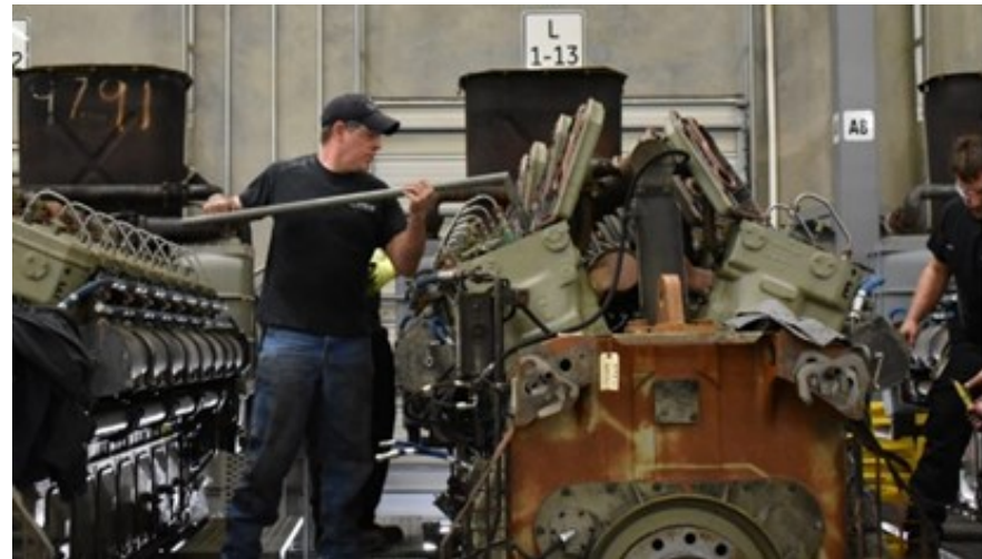
Rebuilding a GE (now Wabtec) prime-mover in Forth Worth. William C. Vantuono photo
