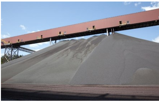
A mountain of low silica DR-grade pellets awaits its journey to Ohio on Tuesday at Northshore Mining. Northshore Mining built a new plant with new equipment to produce low silica DR-grade pellets to be used as feedstock at Cliffs' hot briquetted iron plant in Toledo, Ohio. Ellen Schmidt/
