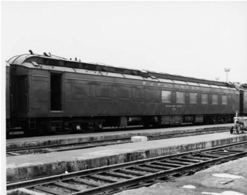
Car 177 on May 16, 1958. This car was equipped with ice activated air conditioning.
