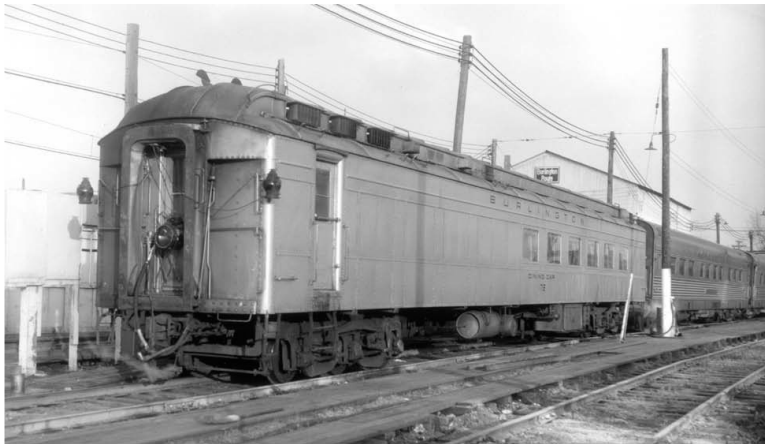
Car 177 on May 16, 1958. This car was equipped with ice activated air conditioning.
