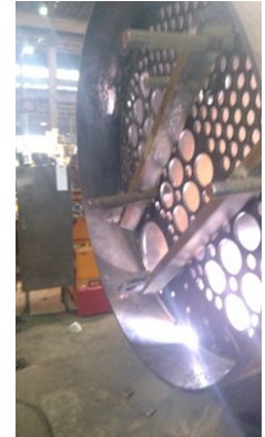
C&NW 1385's new front flue sheet is welded in place. Photo courtesy Gary Bensman
