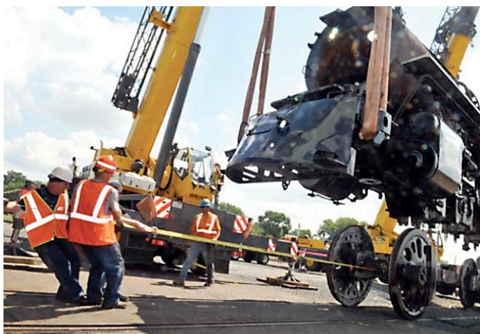
Crews use a winch-powered cable to pull the drivers out from the 261's boiler and frame. Photo by St. Paul Pioneer Press
