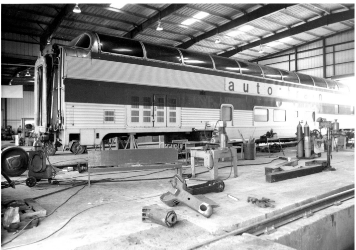
Above: An ex-Santa Fe dome gets "new shoes" during a truck replacement in the Sanford Shop. Photo by Russ Isbrandt
