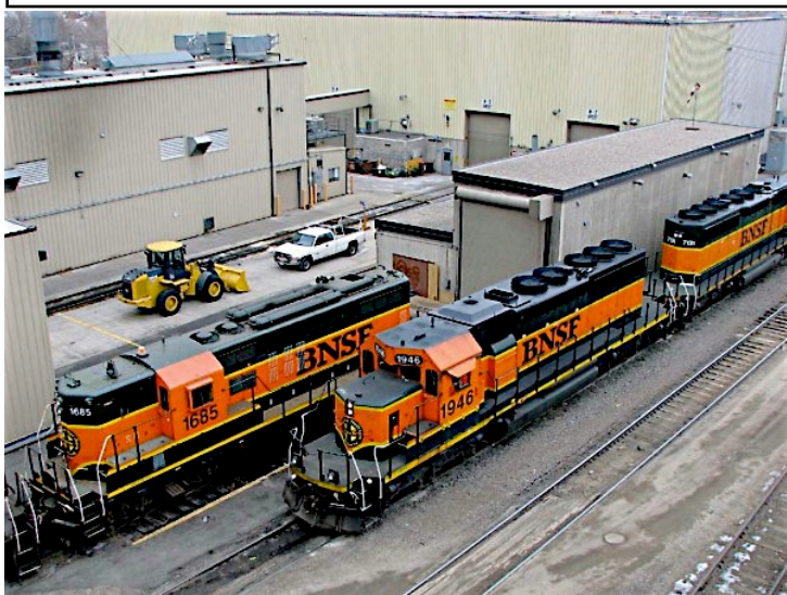
Three BNSF units in Heritage I paint at Northtown, February 13th. The 1685 is of particular interest as it does not have dynamic brakes. It is former BNML (BN of Manitoba) #2 which spent most of its life in Winnipeg. Photo from John Hill collection
