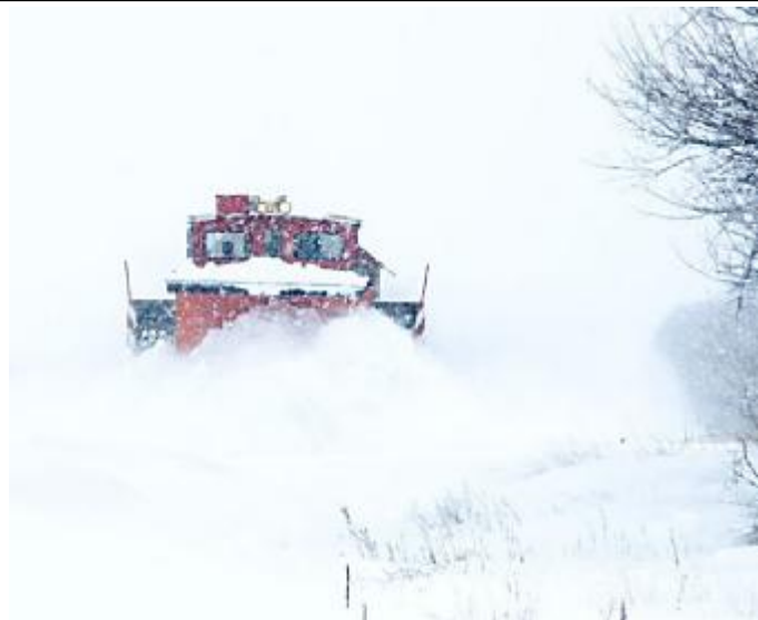
Drift Busters with pneumatically-powered wings extended, CP's plow gets a push from Soo Line SD60 6023 through a drift north of Morrisonville, WI, February 12th. Photo by (TRAINS: Andy Cummings)
