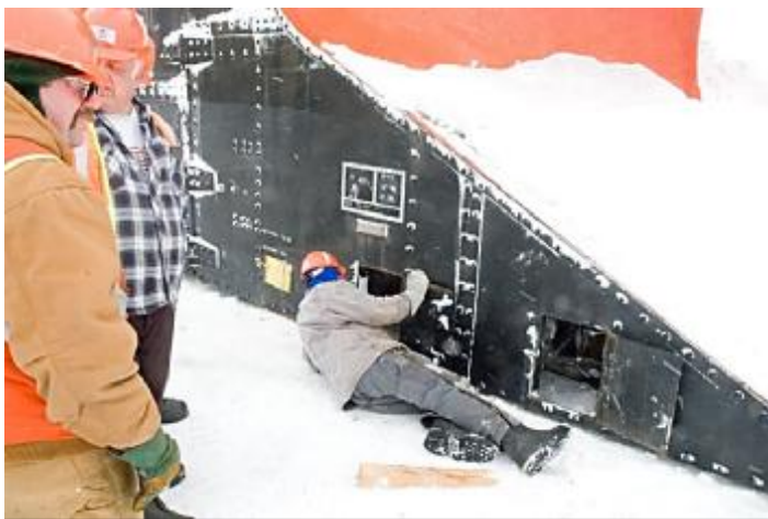
Simple wooden wedges were used to guide the wheels of the wedge plow safely back onto the rails. Photo by (TRAINS: Andy Cummings)
