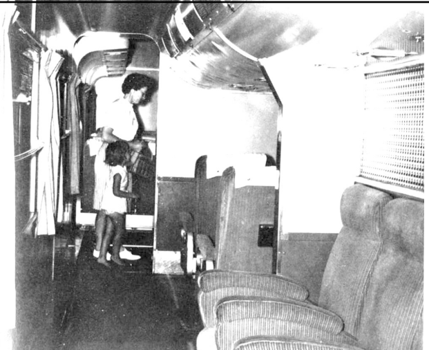
Silver Dome was rebuilt by the Burlington from a regular Budd streamlined coach, Silver Alchemy . This car was configured substantially differently from domes built by Budd. Note the regular reclining coach seats in the dome. Photo below shows the portion of the car beneath the dome. Aisles passed along the outer edges of the car and coach seating was located under the dropped floor of the dome as shown in this photo from Pat Dorin's book, "Everywhere West - The Burlington Route," Superior Publishing, 1976.
