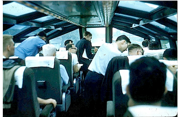
Silver Dome was rebuilt by the Burlington from a regular Budd streamlined coach, Silver Alchemy . This car was configured substantially differently from domes built by Budd. Note the regular reclining coach seats in the dome. Photo below shows the portion of the car beneath the dome. Aisles passed along the outer edges of the car and coach seating was located under the dropped floor of the dome as shown in this photo from Pat Dorin's book, "Everywhere West - The Burlington Route," Superior Publishing, 1976.
