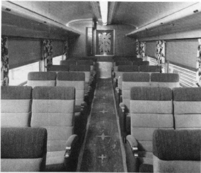
Facing toward the vestibule end of the car (seats are turned opposite from floor plan, top), the center divider can be seen in the background.
