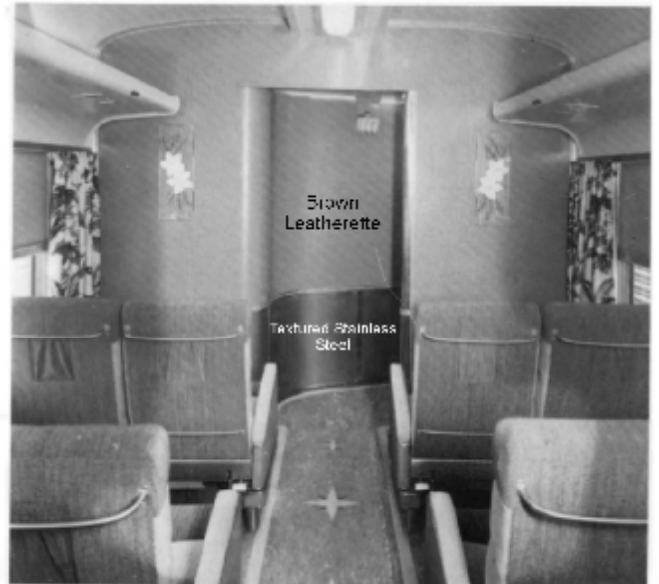
The curved passageways to the restrooms at either end of the car are an innovation. Note star pattern in linoleum—a C&O "signature."
