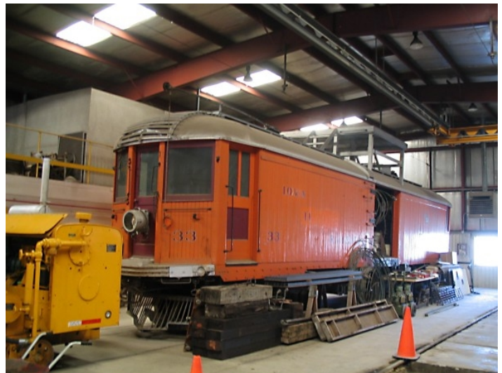
Iowa Terminal line car built from a North Shore merchandise dispatch car. Photo by Russ Isbrandt
